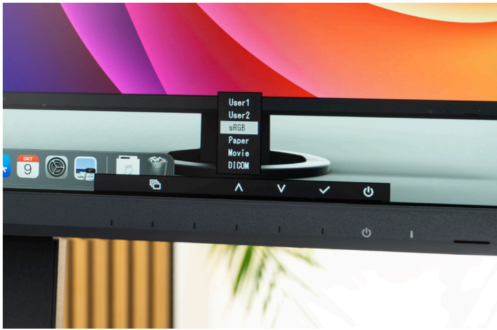
All features can be activated or adjusted with a simple fingertip on the touch-sensitive buttons integrated into the frame.
